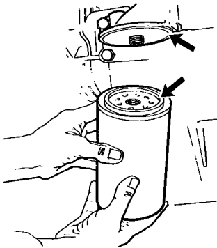
Illustration 68 Typical filter mounting base and filter gasket
